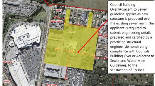
Figure 6: Sewerage Arrangements
