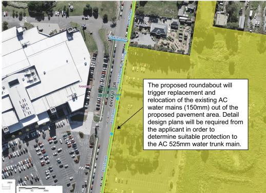
Figure 5: Water Supply Arrangements
