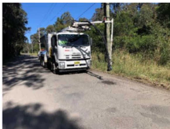
Image: Jet patcher truck, mainly used in less trafficked areas, undertaking small pothole repairs.
