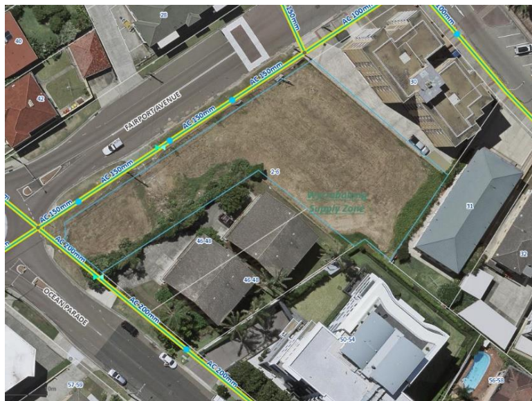
Figure 14: Water servicing arrangements
