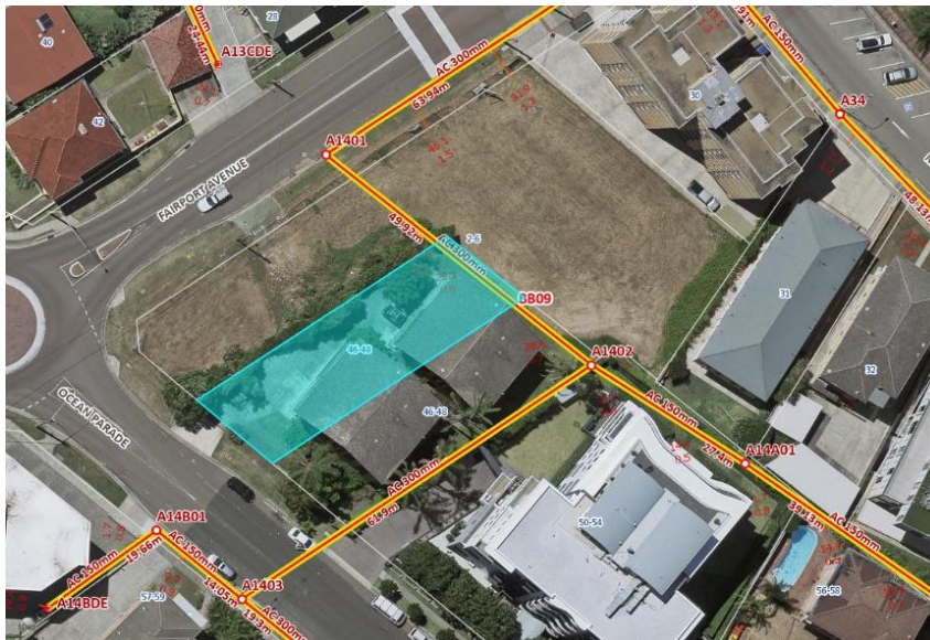
Figure 15: Sewer servicing arrangements
