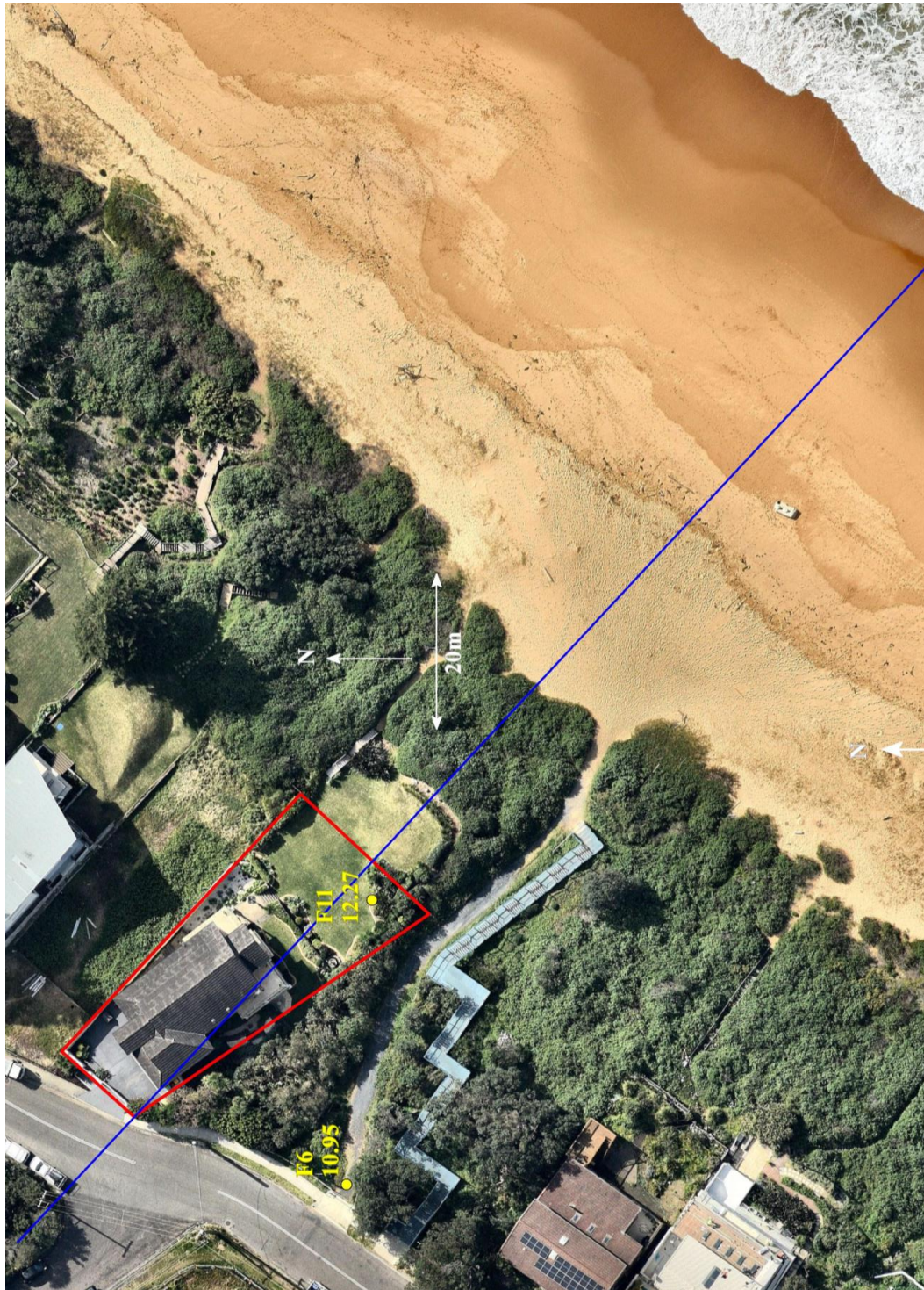
Figure 4: Aerial view of subject property on 18 August 2022, with approximate boundary in red, Coastal & Marine Geosciences (1997) borehole locations and bedrock AHD levels in yellow, and cross section location in blue
