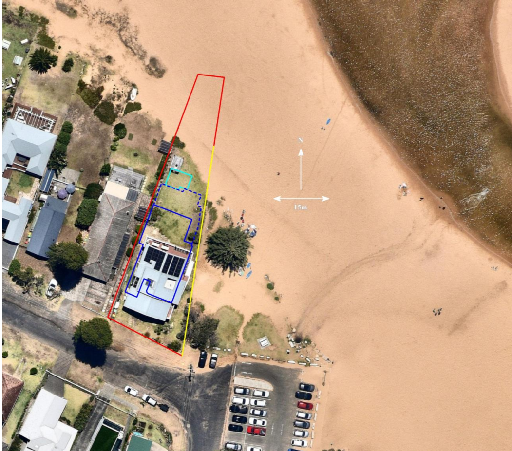
Figure 5: Outline of ground floor of proposed dwelling (solid blue), with outer edge of Terrace 1 dashed blue, proposed Terrace 2 in cyan, proposed wave trip fence in yellow, and approximate site boundary in red (aerial photograph taken 29 October 2023)
