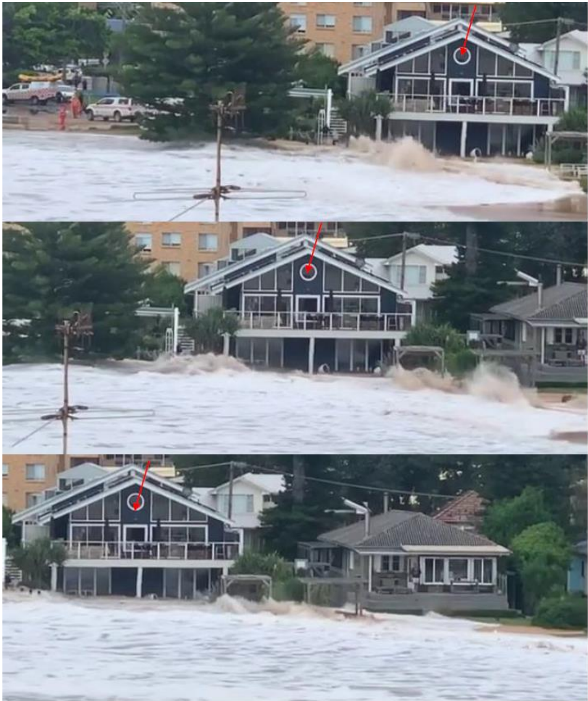
Figure 6: Long-period oceanic inundation event at site in April 2022 (flow from left to right, site at arrow, three images about 3s apart getting later from top to bottom, facing SW)
