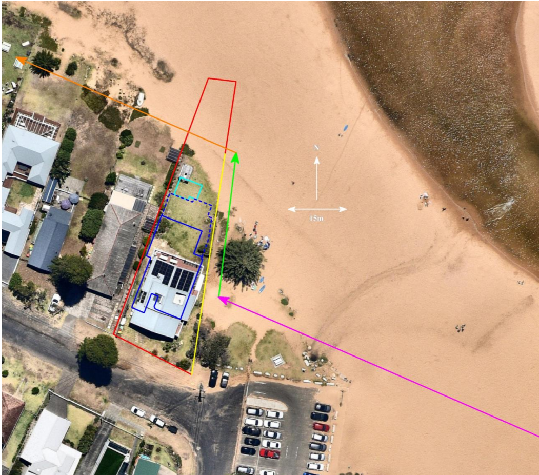
Figure 7: Effect of proposed fence on deflection of oceanic inundation (based on Figure 5, with magenta arrow showing incoming wave energy direction, green arrow showing deflected wave energy direction at the fence, and orange arrow showing deflected wave joining the incoming wave energy direction north of the fence)
