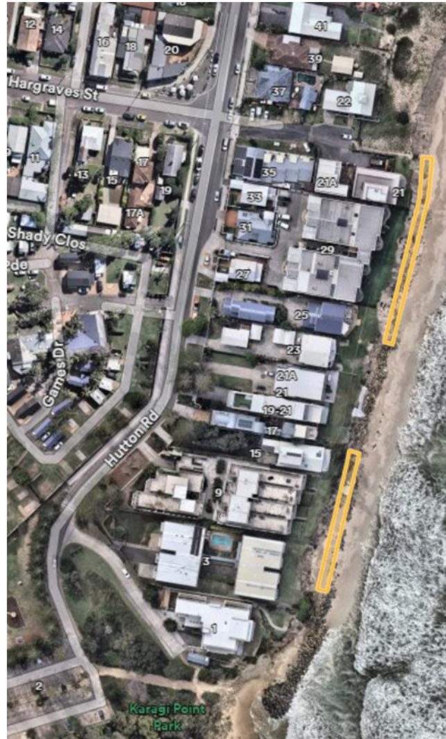
Figure 2: Aerial image of the Entrance North showing areas generally bound by Hargraves Street to the north and Karagi Reserve to the south, with areas highlighted where works may be required to mitigate immediate erosion risks based on preliminary observations by Council staff.
