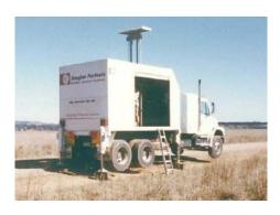
Figure 2: Purpose built CPT rig
